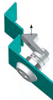
Position 2 Cam will move upright when touches the body
